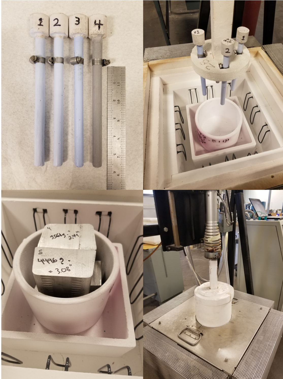
Dynamic melt test set-up at the Edward Orton Jr. Ceramic Foundation. Clockwise from top left: Coated FS73 AL test pins; coated pins inserted into rotating crucible lid; test in progress; and A356 aluminum prior to melting.
